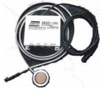
J15D3A Throu-wall Ultrasonic liquid level Gauge is used for fuel level or liquid measurement in vehicle fuel or liquid tanks in order to control fuel consumption. The measurements are realized by the ultrasonic sensor installed directly on the external bottom part of the fuel tank and Mainframe Unit. The Throu-wall Ultrasonic liquid level Gauge can measure levels of diesel and petrol or other liquid materials depending on software settings. Features
