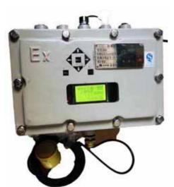
J15D3IB Throu-wall Ultrasonic liquid level meter is used for fuel level or liquid measurement in vehicle fuel or liquid tanks in order to control fuel consumption. The measurements are realized by the ultrasonic sensor installed directly on the external bottom part of the fuel tank and Mainframe Unit. The Throu-wall Ultrasonic liquid level meter can measure levels of diesel, Acids / solvents and petrol or other liquid materials depending on software settings. Typical ATEX Ultrasonic Sensor.
