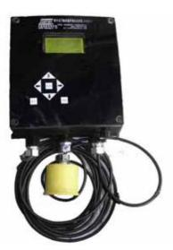
J15D3II Throu-wall Ultrasonic liquid level meter is used for fuel level or liquid measurement in vehicle fuel or liquid tanks in order to control fuel consumption. The measurements are realized by the ultrasonic sensor installed directly on the external bottom part of the fuel tank and Mainframe Unit. The Throu-wall Ultrasonic liquid level meter can measure levels of diesel, Acids / solvents and petrol or other liquid materials depending on software settings.
