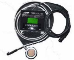
J15D3C Throu-wall Ultrasonic liquid level Gauge is used for fuel level or liquid measurement in vehicle fuel or liquid tanks in order to control fuel consumption. The measurements are realized by the ultrasonic sensor installed directly on the external bottom part of the fuel tank and Mainframe Unit. The Throu-wall Ultrasonic liquid level Gauge can measure levels of diesel and petrol or other liquid materials depending on software settings.
